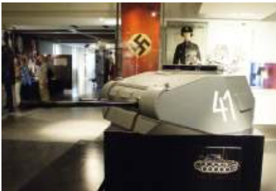
Turret of a German Mark II tank, equipped with a 2 cm gun and a MG.
