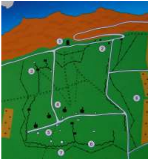
Ground plan of WN 48 with 1) the fire control, observation and command post, 2) a Tobruk, 3) store for ammunition, 4) the combat bunkers, 5) store for ammunition, 6) trenches, 7) barbed wire and 8) minefields (Source: Desquesnes page 22)
